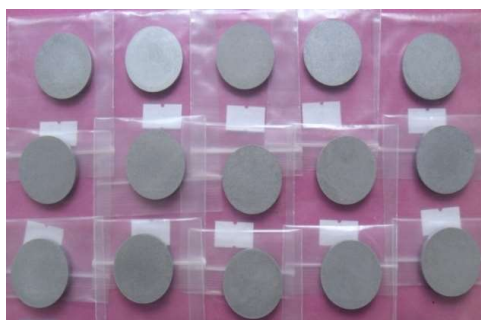
Figure 1. The photograph of pressed pallets of aluminum dioxide samples
