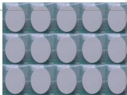
Figure 2. The photograph of pressed pallets of silicon dioxide samples
