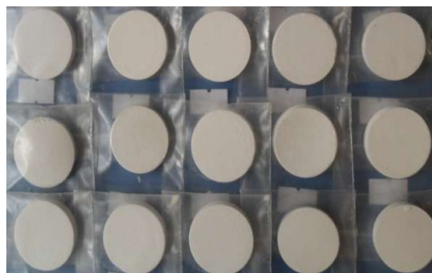
Figure 4. The photograph of pressed pallets of potassium carbonate samples
