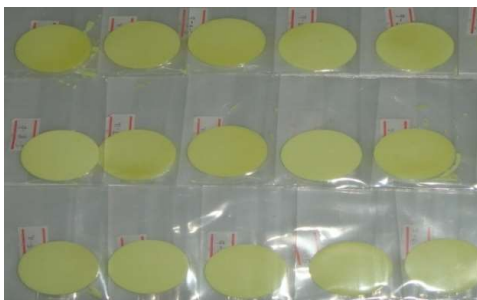
Figure 3. The photograph of pressed pallets of sulfur samples
